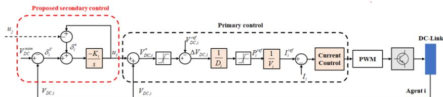
Fig. 2 Overall block diagram for the proposed control scheme.
