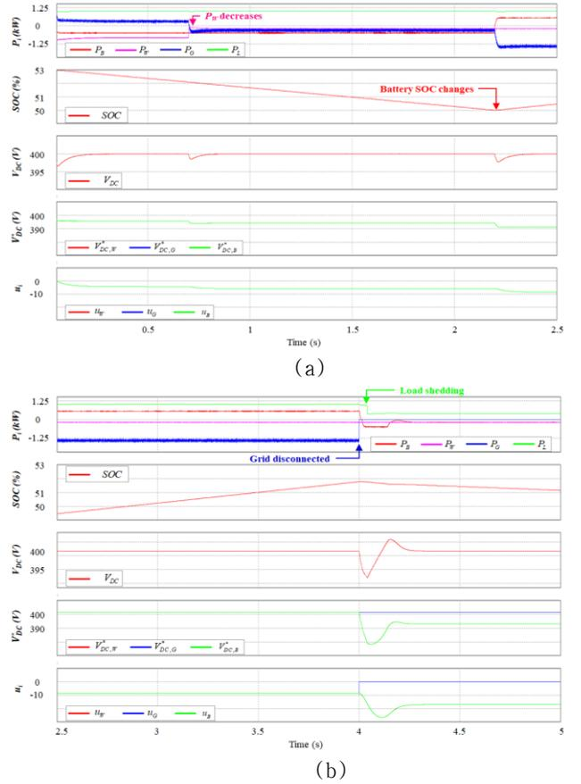
Fig. 4 System responses under various conditions. (a) In grid-connected mode. (b) Transition from grid-connected mode to islanded mode.
