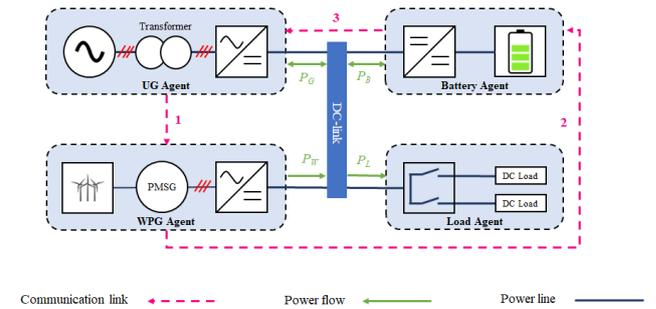
Fig. 1 Configuration of the proposed distributed DCMG.
